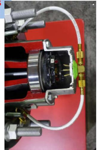
The inflation system can keep the tires properly inflated by using compressed air from the trailer's air system to inflate any tire that falls below a preset pressure whenever the vehicle is in operation.
